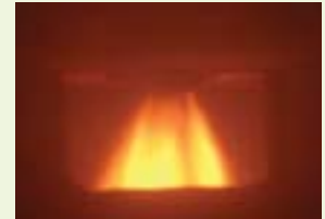
b) Lignite/air flame with 3 volume-percent oxygen excess
