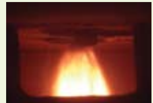
b) Lignite/air flame with 3 volume-percent oxygen excess
