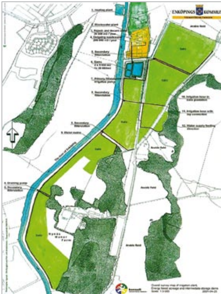
Figure 9. Plan of the area with the heating plant, sewage purification plant, and adjacent Salix plantations which are utilised for sewage water treatment.
