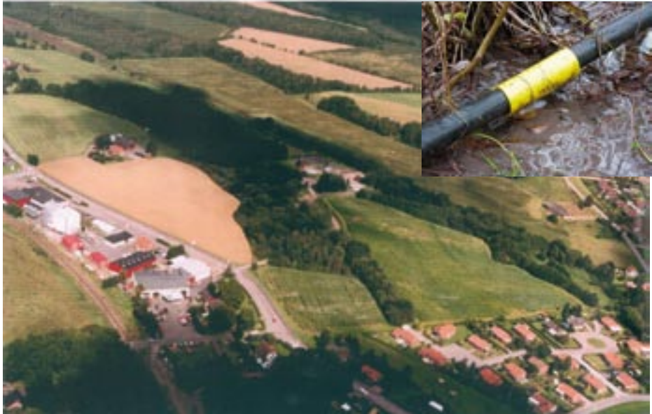
Figure 7. View over Kågeröd in Svalöv municipality, where Salix plantations are irrigated with pre-treated sewage water from the local purification plant. The inset picture shows a detail of the drop-irrigation hoses that are used in the facility. (Photo: Kenth Hasselgren, SWECO VIAK AB.)
